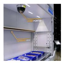
To meet the customer's requirement of reduce space and fast efficient retrieval of goods, 6 units of 12.1m vertical lifts were build in replacement of the racking. To assist and increase picking efficiency, assisted picking accessories were added on each of the vertical lifts. This includes the laser pointer and Alphanumeric Bar. Assisted Put-to-light carts / trolley were also customized and build to assist the operator in picking.
